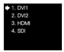
In the cropping setting submenu of **HDMI**, **DVI1**, **DIV2** or **SDI**, press the knob/**OK** to turn the cropping function on or off. If **Enable** has been switched on, you can rotate the knob to set the row starting point (**X**), column starting point (**Y**), and the width and height of the signal image, and then select **Save**.
