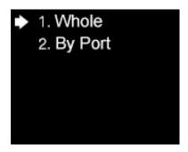
Output shift contains two selections: **Whole** and **By Port**. On the submenu of **Whole**, you can rotate the knob to set the row starting point (**X**) and the column starting point (**Y**) of the whole image and then save the setting; on the submenu of **By Port**, you can respectively set the row starting point (**X**) and the column starting point (**Y**) of the image of the 6 Ethernet ports, and then save the setting.
