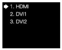
In the EDID setting submenu of **HDMI**, **DVI1 or DVI2**, you can rotate the knob and select a conventional resolution to save the selected resolution to the sender, or select **Custom** and set the width, height and frame rate, and then select **Save** to save the setting to the sender.
