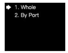
Output shift contains two selections: **Whole** and **By Port**. On the submenu of **Whole**, you can rotate the knob to set the row starting point (**X**) and the column starting point (**Y**) of the whole image and save the setting; On the submenu of **By Port**, you can respectively set the row starting point (**X**) and the column starting point (**Y**) of the image of the 4 Ethernet ports and save the setting.
