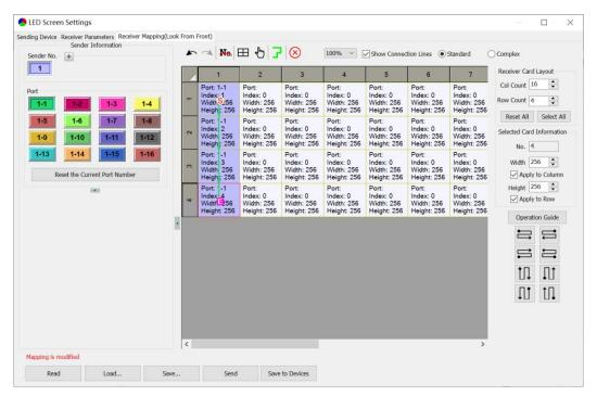
For the cabinets with different specifications (different in dimensions), you can select them and adjust the mapping separately after setting.
