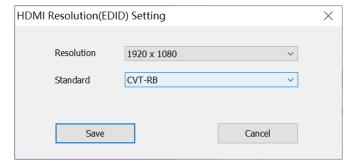
Click the dropdown button. From the resolution list, you can select a conventional resolution, or select **Custom** and set the width, height, frame rate and standard of the customized resolution.
