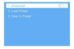
In the submenu, you can turn the **Broadcast** function on or off, and save 16 preset parameters, every one of which includes the following parameter information: scaling, cropping, multi-window display, picture adjustment and 3D. You can also directly load the saved preset parameter to display the image based on your specific need without the need to setting the parameters of video sources again. After restoring factory settings, 4 preset parameters have been preset in the controller.
