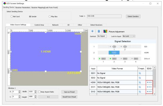
In the **Resolution (EDID) Setting** dialog box, the resolution of the current sender is displayed by default.
