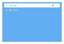
Output shift includes two selections: **Whole** and **By Port**. On the submenu of **Whole**, you can rotate the knob to set the row starting point (**X**) and column starting point (**Y**) of the whole image and save the setting; On the submenu of **By Port**, you can respectively set the row starting point (**X**) and column starting point (**Y**) of the image of the 16 Ethernet ports and save the setting.
