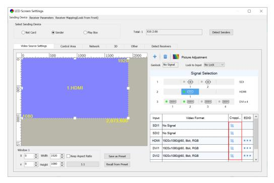
In the cropping setting window, select the **Cropping** check box, and set the row starting point (**X**), the column starting point (**Y**), and the width and height in the **Cropping Settings** area.
